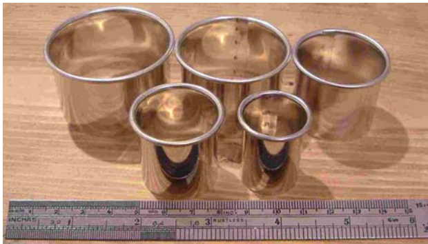
Fig. 2 Stainless steels cylinders used in the hot cutting method
